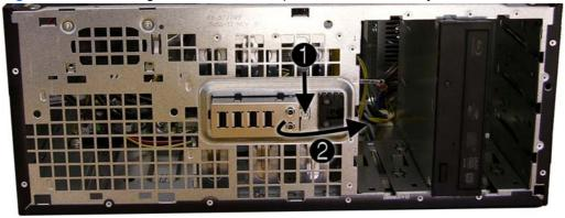
Figure 5-37 Removing the front I/O, USB, power switch assembly
